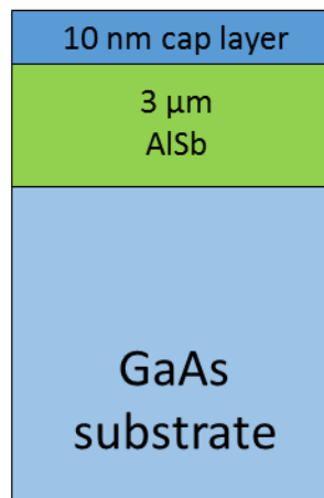
Figure 48. AlSb doping study sample structure.
